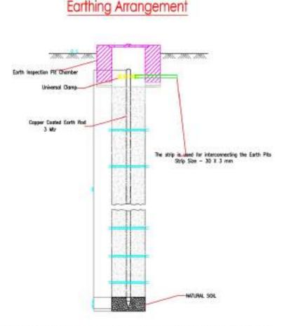
Note: we have to auger the soil up to 1mir with 100 mm dia and fill up the pit with the 25 kg compound.
